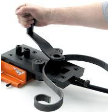
Fig. 7 Rolling Process using portable machine
