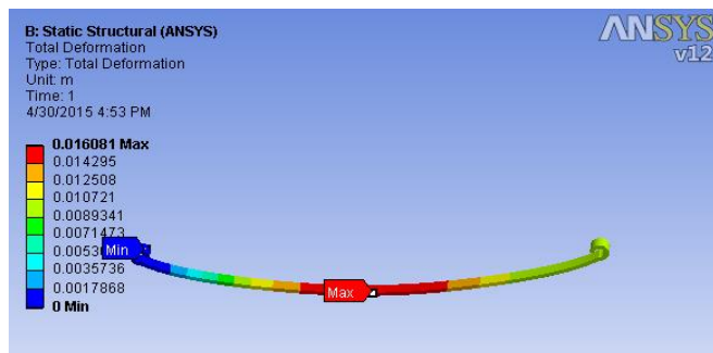
Fig. 8. Total deformation of composite leaf
