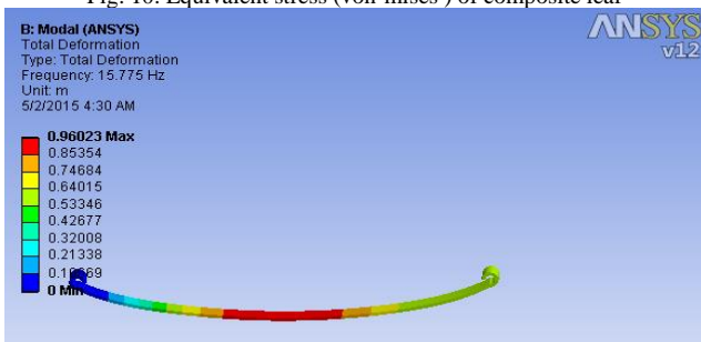
Fig. 11. First natural frequency of composite leaf
