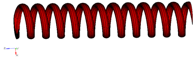
Fig 4.4. Meshed model of Suspension Spring
