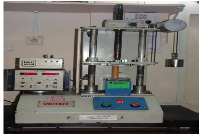
Fig 5.1. Experimental set up of suspension spring
