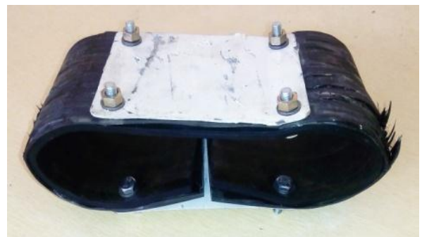
Figure 7 Fracture of elliptical leaf spring with CFRP material during test at 4650N
