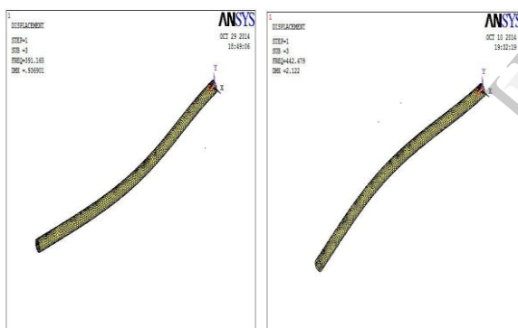
Fig 4.4 Comparison of third set of natural frequency analysis for steel and composite
