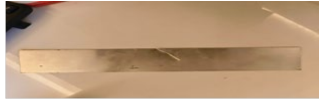
Figure 7. Aluminum Sheet with Crack at center
