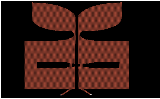
Fig.8. Circular Aperture Patch Antenna With a Common –mode noise Rejection Filter.
