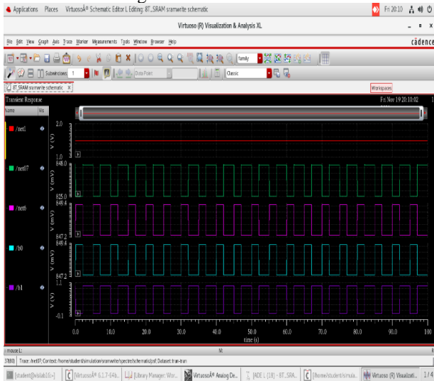
Figure 4: 6T SRAM cell Write Operation
