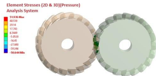
Figure 18 Case III-1.5kW- Pressure distribution on Stainless Steel
