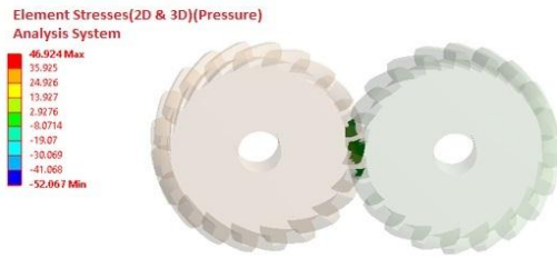
Figure 21 Case III-1.5kW- Pressure Distribution on Nylon 66
