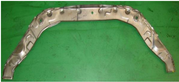
Fig 2: Cross member panel with heavy wrinkling defect.
