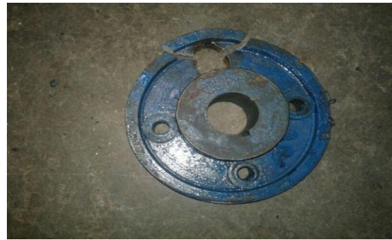
Fig-3 Coupling Broken
