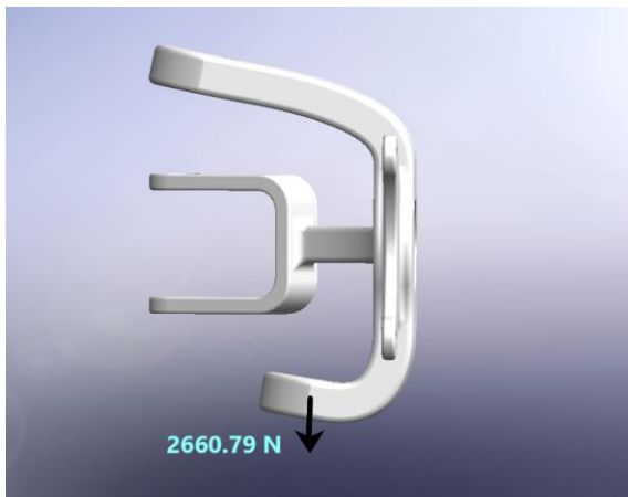
Fig 15. Knuckle side view, Force due to bump
