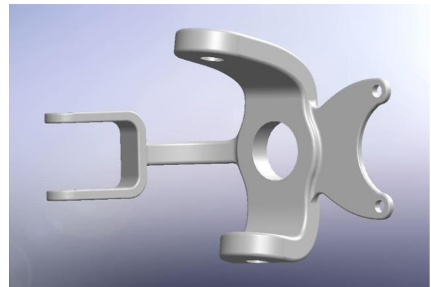
Fig 13. The final design of the knuckle
