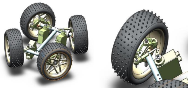
Fig 2 . Zero Turn Mode and Components Assembly
