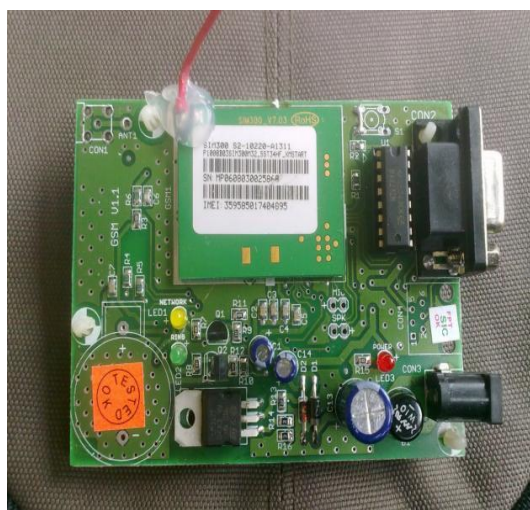
Fig.9: Fabricated circuit of power supply, MCU and GSM
