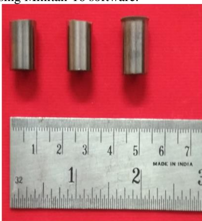
FIG.1. WC/CU CYLINDRICAL ELECTRODE FOR EDC
