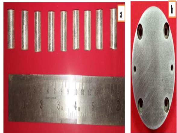
FIG.2. A) WEAR TEST SPECIMEN B) COUNTERPART DISC (EN31 STEEL)
