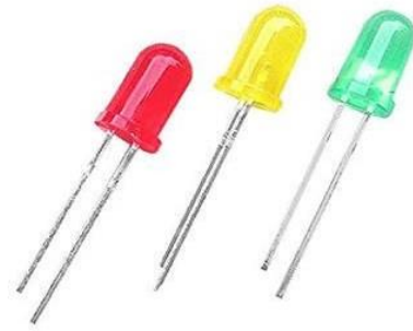
Figure 6: Light Emitting Diode.
