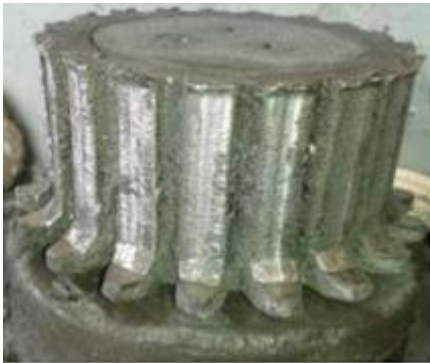
Fig. 6. Pinion Completely Worn out [4]
