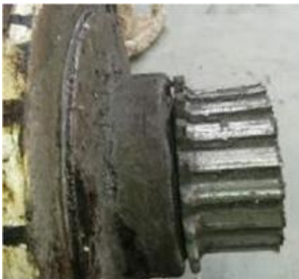
Fig. 7. Dirt around the Pinion [4]
