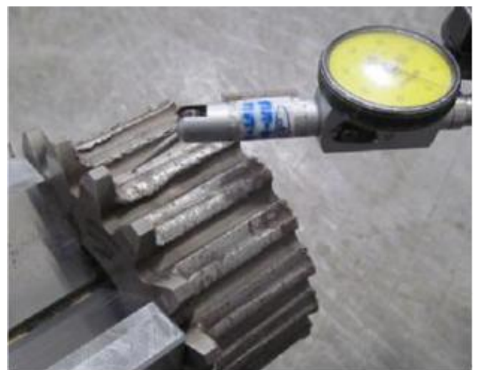
Fig. 10. Depth of Wear Measurement [5]
