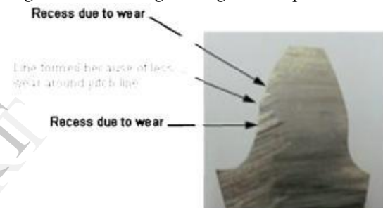
Fig. 9. Pinion with Line near the Pitch Line [5]
