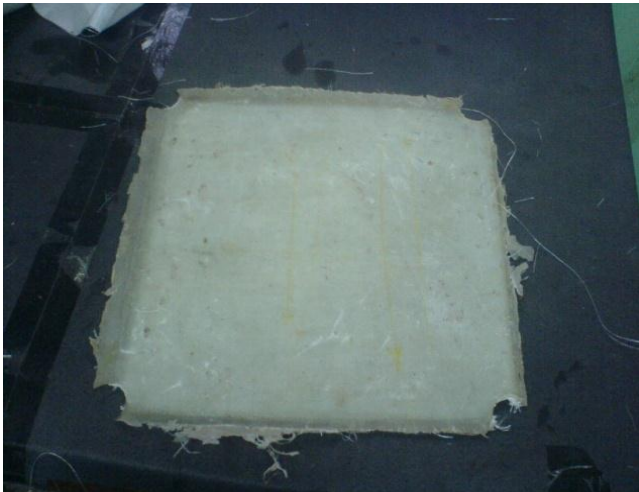
Fig.1 GFRP Cross ply laminate after curing from Compression Moulding Machine
