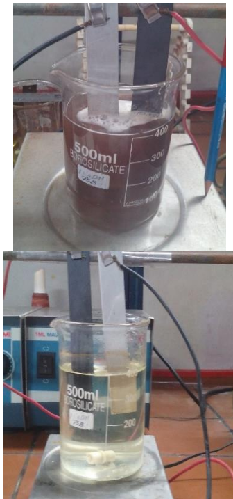
Figure 15 Raw and decolourised Reverse Osmosis Reject
