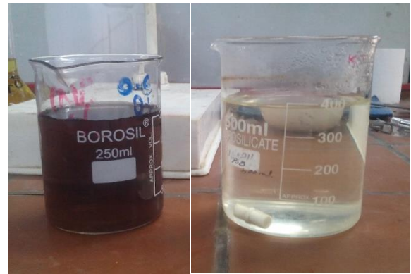
Figure 8 Raw and decolourised secondary treated effluent
