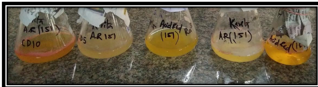
Fig. 2: Decolorization of Acid Red 151 after 7 days of inoculation in all the five bacterial cultures.
