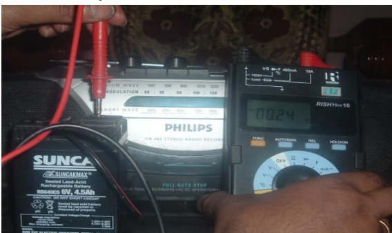
Fig 6: Radio cum tape recorder powered by 4.5AH battery charged from 12V, 75AH battery.
