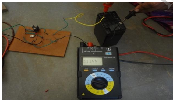
Fig 5: Battery of 6V, 4.5AH charged by 12V, 75AH battery.
