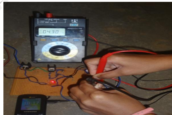
Fig2: Output voltage of prototype charger
