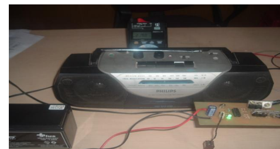
Fig 9: Radio running with inverted square wave ac output.
