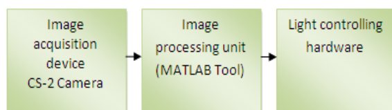
Figure2: Block diagram of daylight sensing and processing unit
