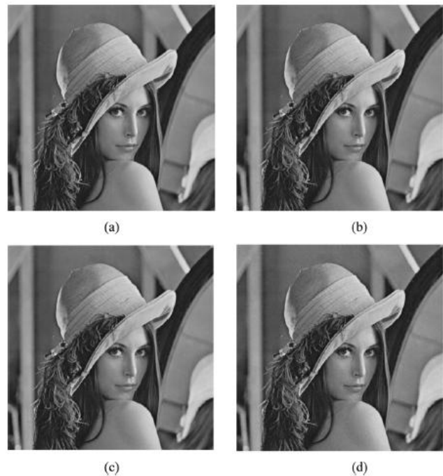
Fig. 5. Cover image and stego images under various payloads. (a) Cover image. (b) Stego image, 2 bpp at 46.86 dB. (c) Stego image, 3 bpp at 40.97 dB. (d) Stego image, 4 bpp at 34.90 dB.
