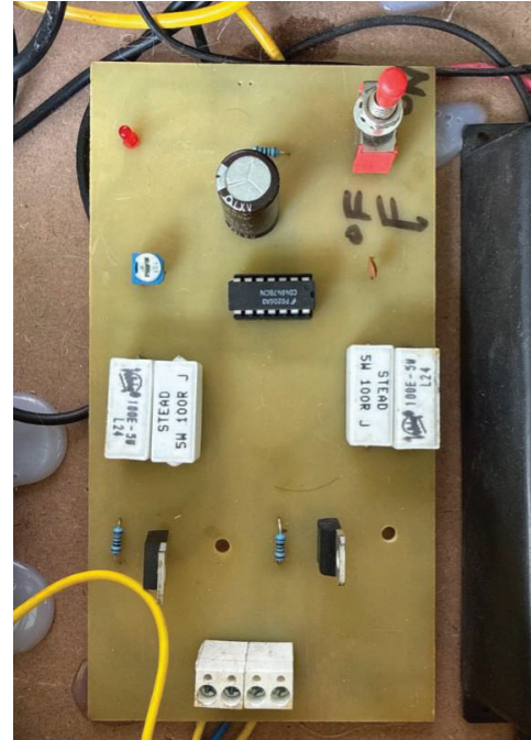
Fig. 3. CD4047 oscillator circuit configured for 50Hz square wave generation with complementary outputs for MOSFET driver.
