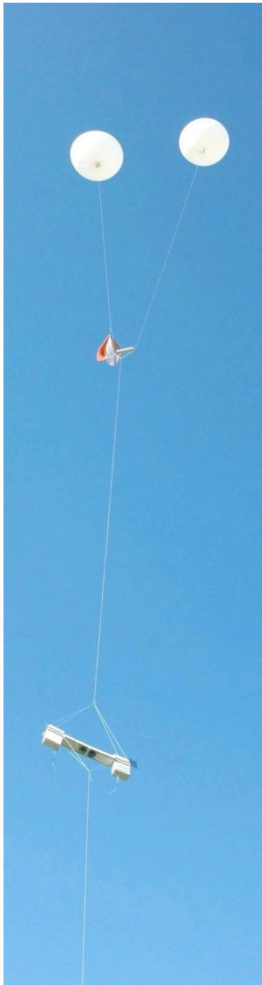
Figure 8. Flight configuration for the double balloon method. Each of the two balloons and payload are attached to a vertex of a triangular aluminium frame outfitted with the Intelligent Balloon Release Unit that releases the carrier balloon at a preset altitude. The configuration is shown attached to the launching pole just prior to release.
