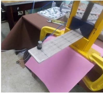
Fig 22: Fixing of accelerometer
