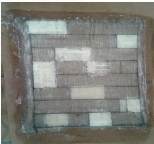
Fig 12: Plying up with suitable adhesives
