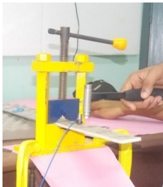
Fig 23: Striking with impact hammer
