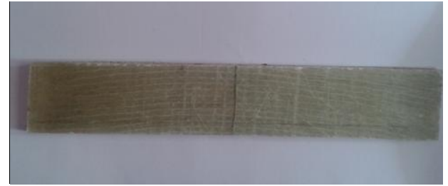
Fig. 14: Specimen without delamination
