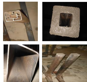
Figure . 1. Test specimen SQ-1 and control specimen CS-1 before and after concreting
