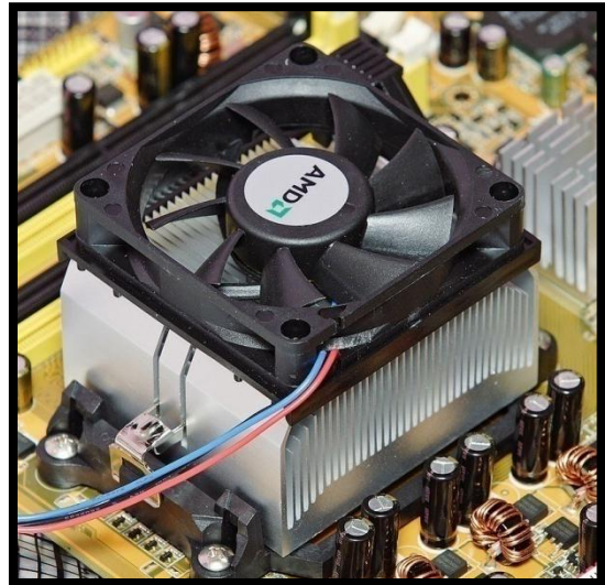
Fig.1 Aluminium heat sink for conventional air cooling
