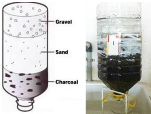
Fig. 3: Constructed Low Cost filter
