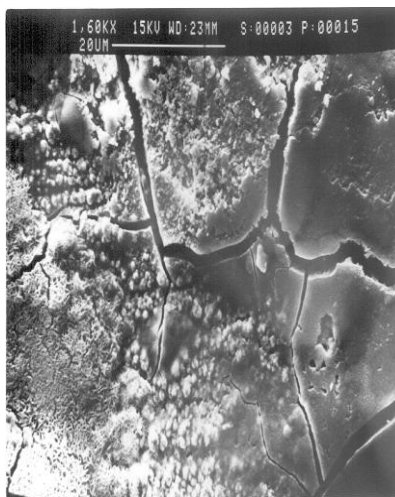
Fig. 11: SEM micrograph of L-80 grade steel in H 2 S medium
