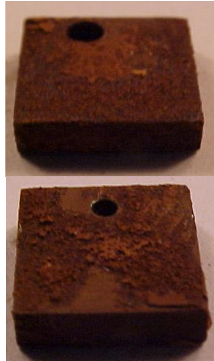
Fig.7: Physical appearance of exposed samples (a) CO_2 and (b) H_2S medium
