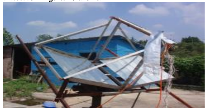
Figure 15. Setup of passively cooled CPV using water. [10]
