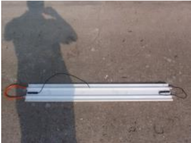
Figure 16. Water channel used for CPV cooling. [10]
