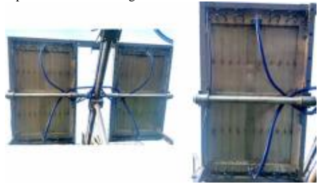
Figure 14. Setup of passively cooled PV panel and water heating configuration. [16]
