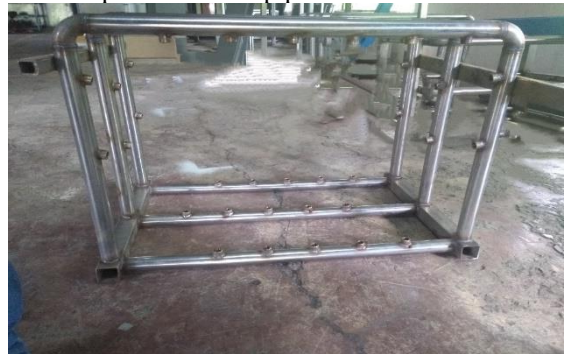
Figure no. 8. Fabrication of Nozzle Tree
