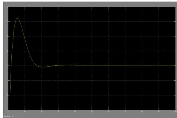
Previous graph is open loop system graph. Now a controller called PID controller is used to control the system which is in closed loop. Thus the output graph is obtained by using a controller called PID controller. The graph is got by comparing the values of Zn-II tuning method. After that manual tuning is done and the output is obtained. The resulting output is shown below.
