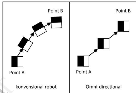
Figure 5. The difference of Wheel Conventional and Omni-directional Wheel
