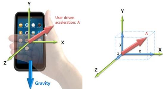
Figure 4. Coordinate System of Smart-phone
