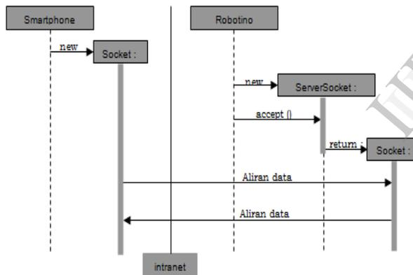
Figure 2. Communication Process of Smart-Phones with Robot
