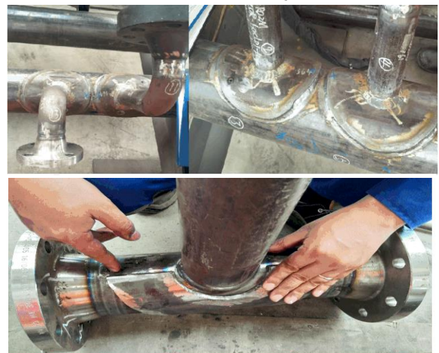
Fig. 6. R-pads are too close to adjacent welds, raising local stresses, restricting welding/NDE access, and risking nonconformance/rework
