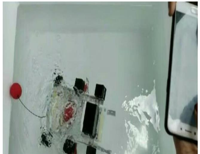
Fig. 3. ROV in pure water
