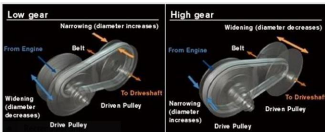
Fig 2: Working of CVT
