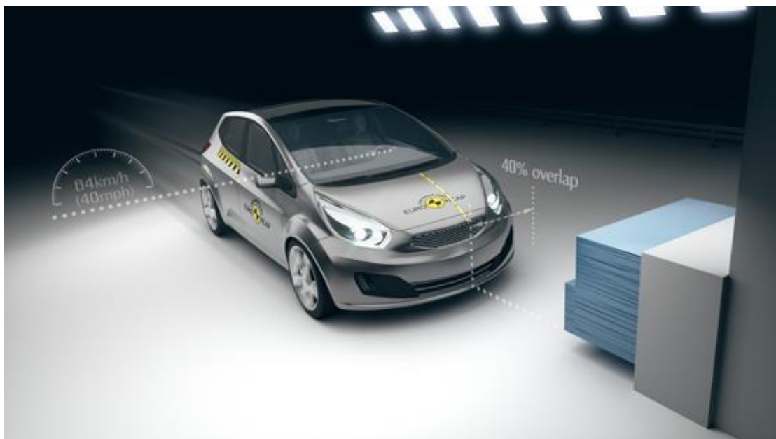
Figure 1.2.2 Frontal offset crash test
