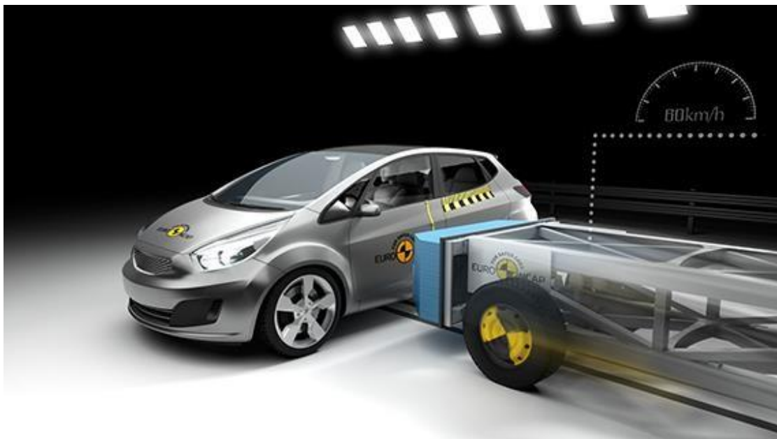
Figure 1.2.3 Side impact crash test
