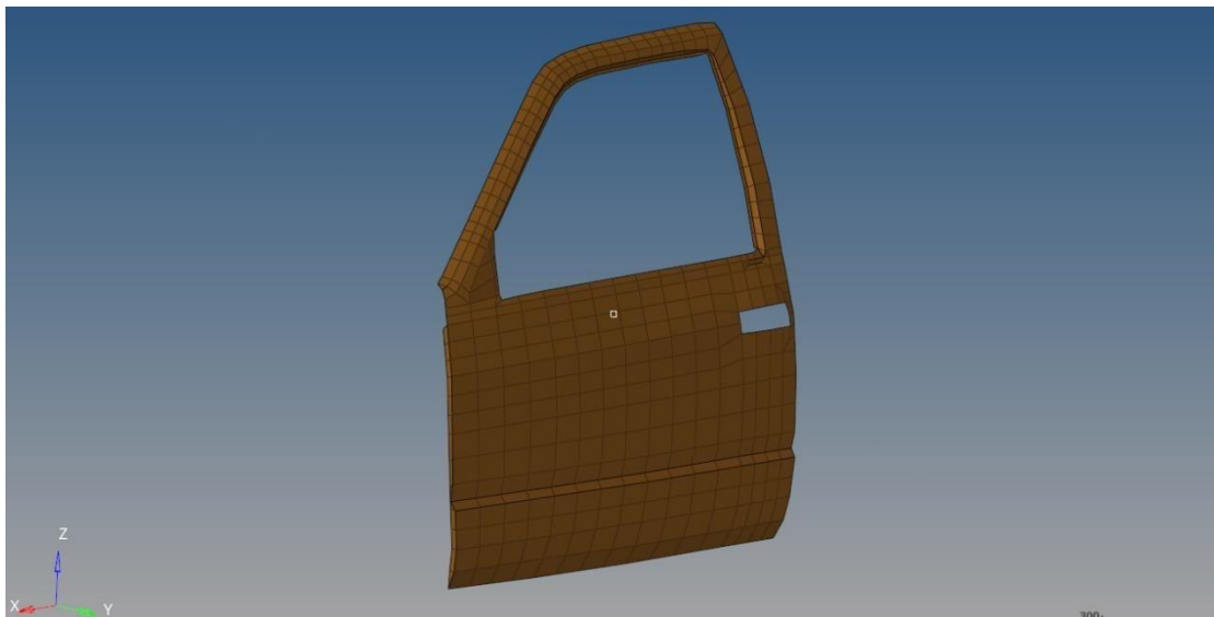
Figure 4.4.2 Door 2D mesh
