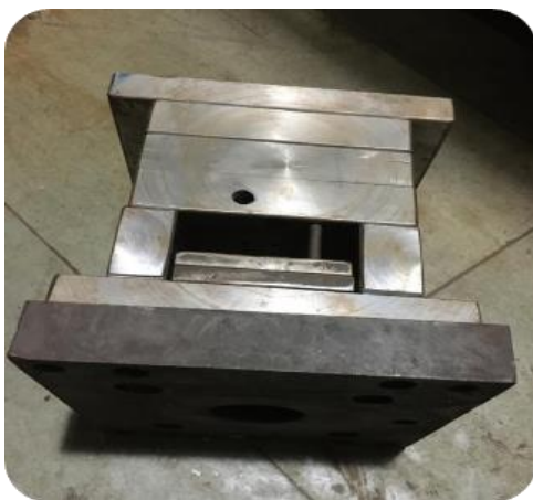
Fig. 8. Mold after machining and polishing.
