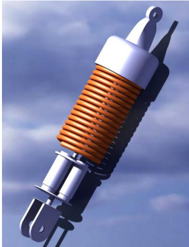
Fig IV. (e) Shown describes maximum load condition with full suspension travel
