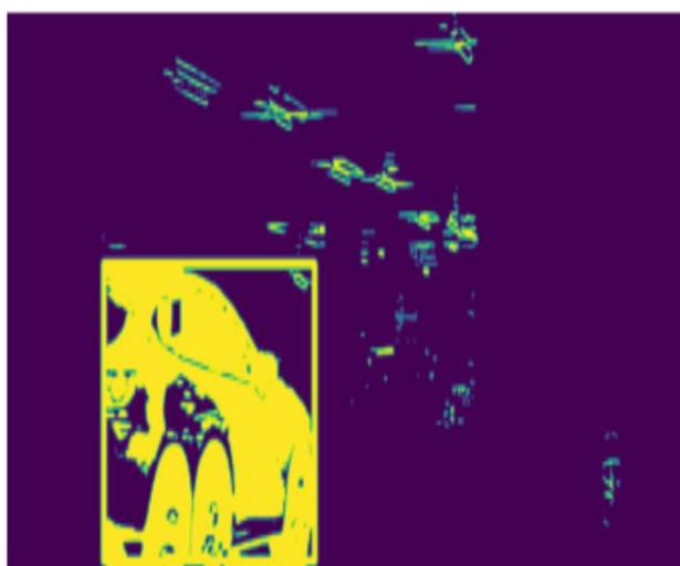
The threshold for the area of the contour has been set to one lakh so that unnecessary small contours and the frames containing small partial images of the car are not counted.
