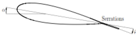
Fig. 2 Airfoil cross section and serrated trailing edge flap. Angle of attack, \alpha , and the serration flap angle, \phi , are shown
