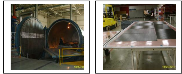
Figure 5. Autoclave used for heating and tool for prepregs
