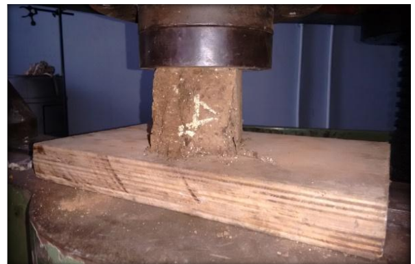
Fig. 2: Compression Test on Block
