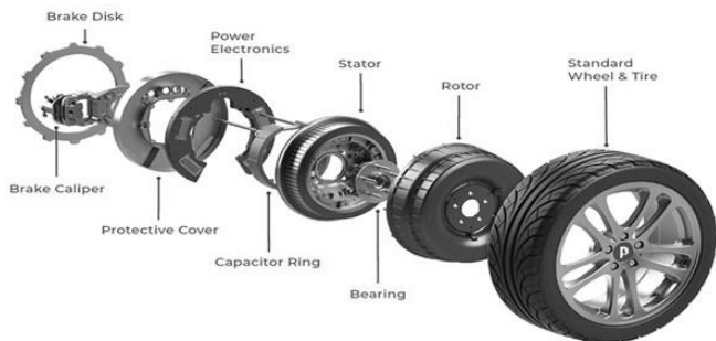
Fig.4 View of In Wheel Drive System in EV
