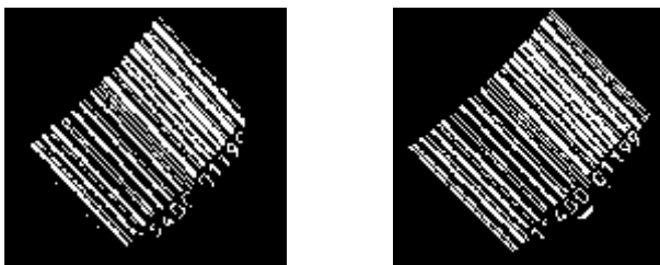
Result using Juett and Qi's Method Result using Tuinstra's Method Fig. 16: Results of algorithms on images having skewed barcodes
