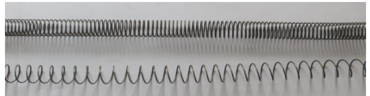
Figure no. (5) Sample Coiled Inserts (Circular and Square Cross-section with different pitch)
