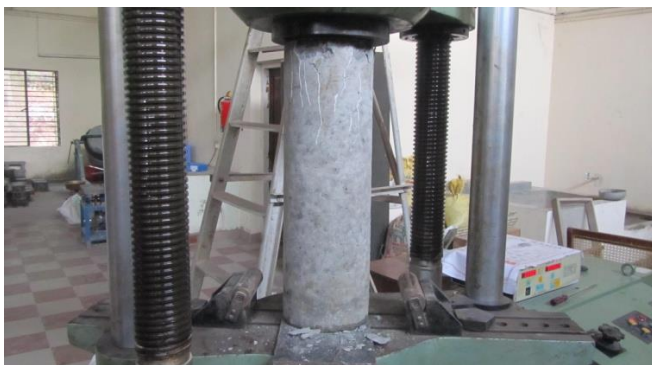
Fig. 4. Compression testing of column
