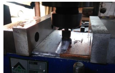
Fig.1 Friction stir welding process
