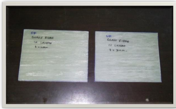
SPECIMENS- GLASS EPOXY LAMINATES
