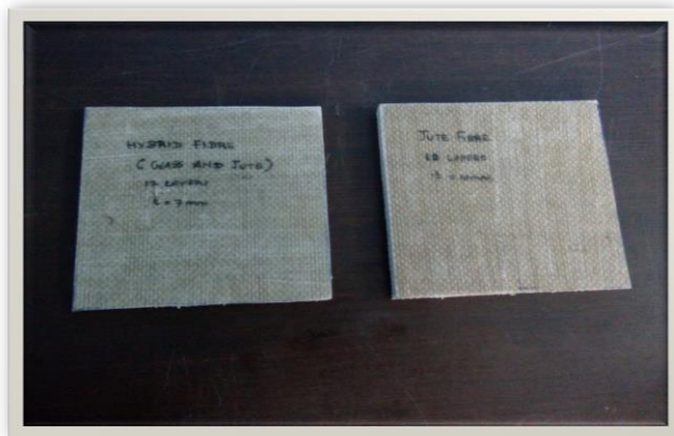
SPECIMENS- HYBRID AND JUTE LAMINATES
